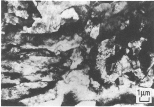
Figure 2 A thin foil micrograph of the specimen quenched from 1100°C, showing a massive martensitic structure.
