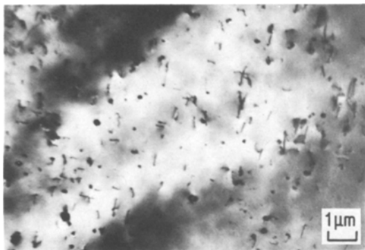
Figure 5 A thin foil micrograph of the specimen annealed at 900°C for 1 h, showing many precipitates which could not be identified.
